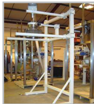
Volumetric filling of dust-free, free-flowing granular materials.
