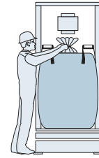
8. Bulk bag spout removed from filling nozzle & tied
